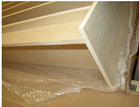
Figure 9. Modified QRD-diffuser, side pane is missing.
