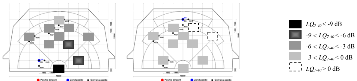
Figure 6: Stage E - overview of results for LQ_{7-40} for source S4 (left) and source S1 (right).
